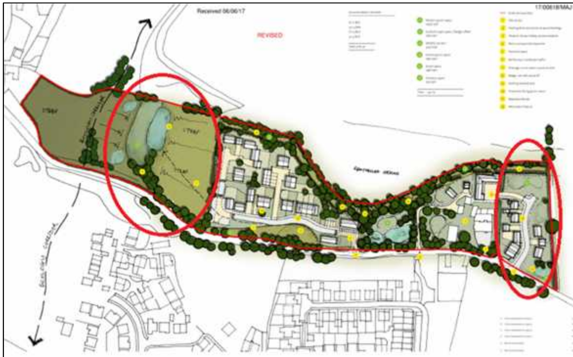
Figure 2: Illustrative Site Layout as submitted by the applicant illustrating how the development areas have swapped due to the topography of the land.
